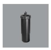
34974.000 Distribution box, IP68 With four cable entries, 7-25mm. Polymer. Ø 102mm, L 305mm. Weight 0.47kg € IP 68 3m
